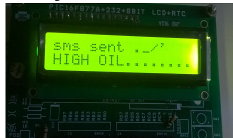
Sms received: transformer oil level is high!!!!!!
