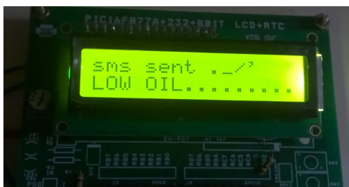
Received message:transformer oil level is low!!!!!!
