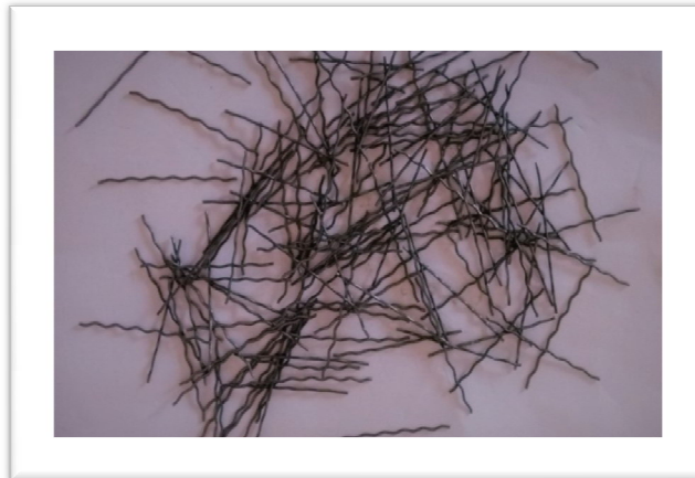
Fig 6 : Crimped steel Fibers
