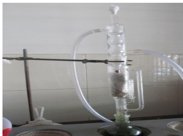
Fig.2. Solvent extraction by soxhlet apparatus
