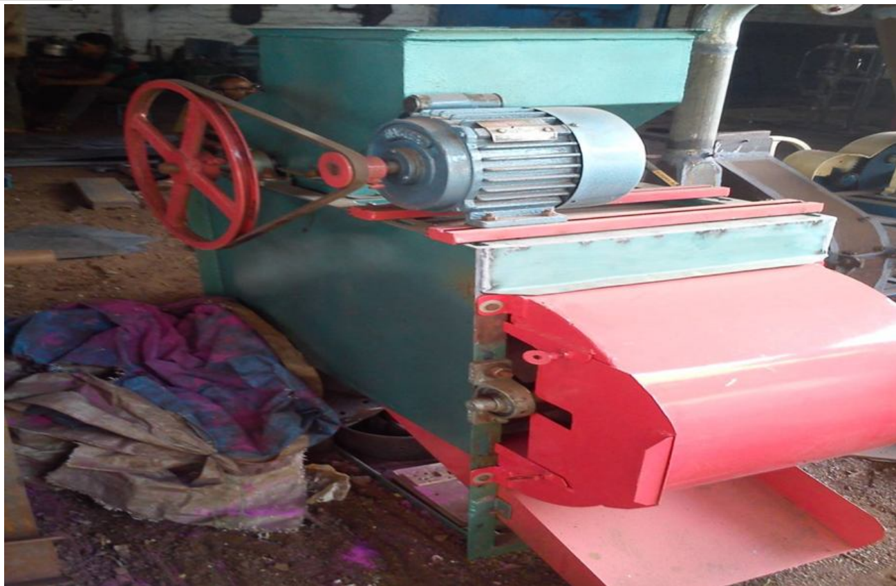
Photo 1 Final Assembly of Groundnut Decorticator
