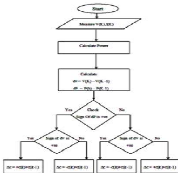
Fig.4 Flow chart of Modified P&O algorithm
