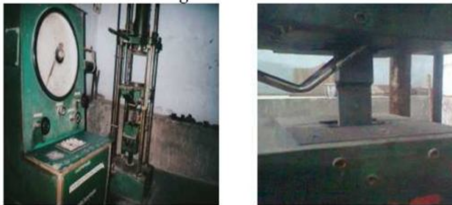
Fig. 2: mounting and loading of test specimen on UTM
