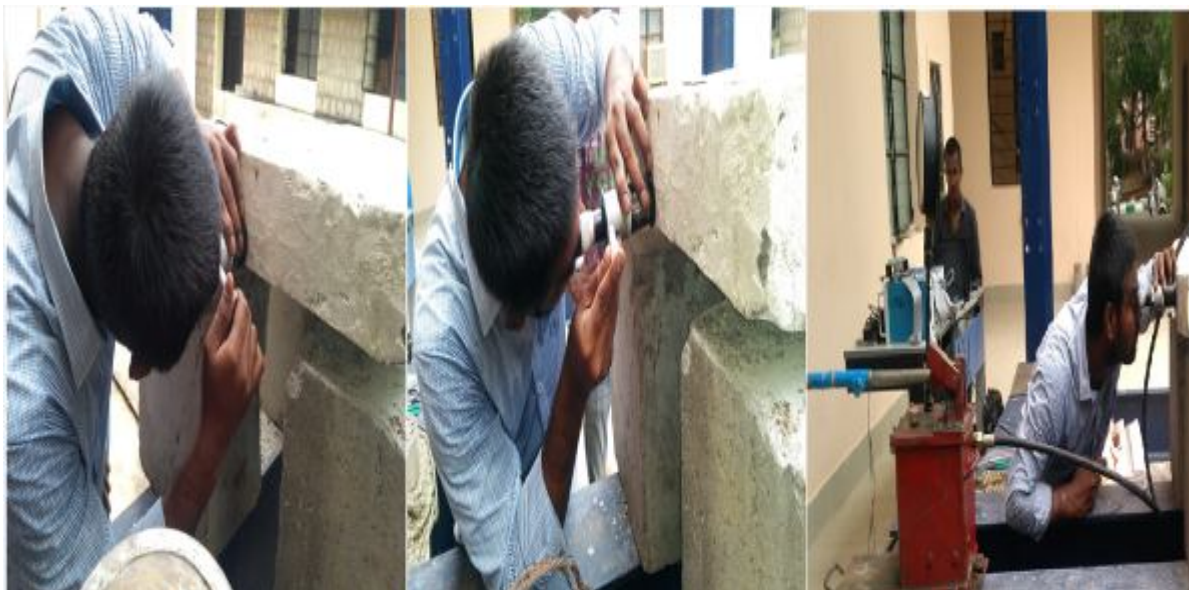
Fig 8: Crack width observation of slab specimens
