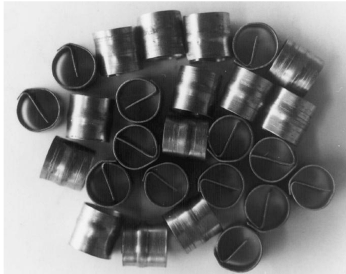
Fig. 3 photographic view of the lessing rings (Velraj et al. [15])
