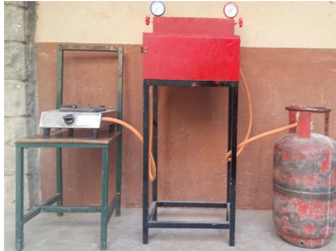
Fig.-2: Actual Setup of LPG Refrigerator
