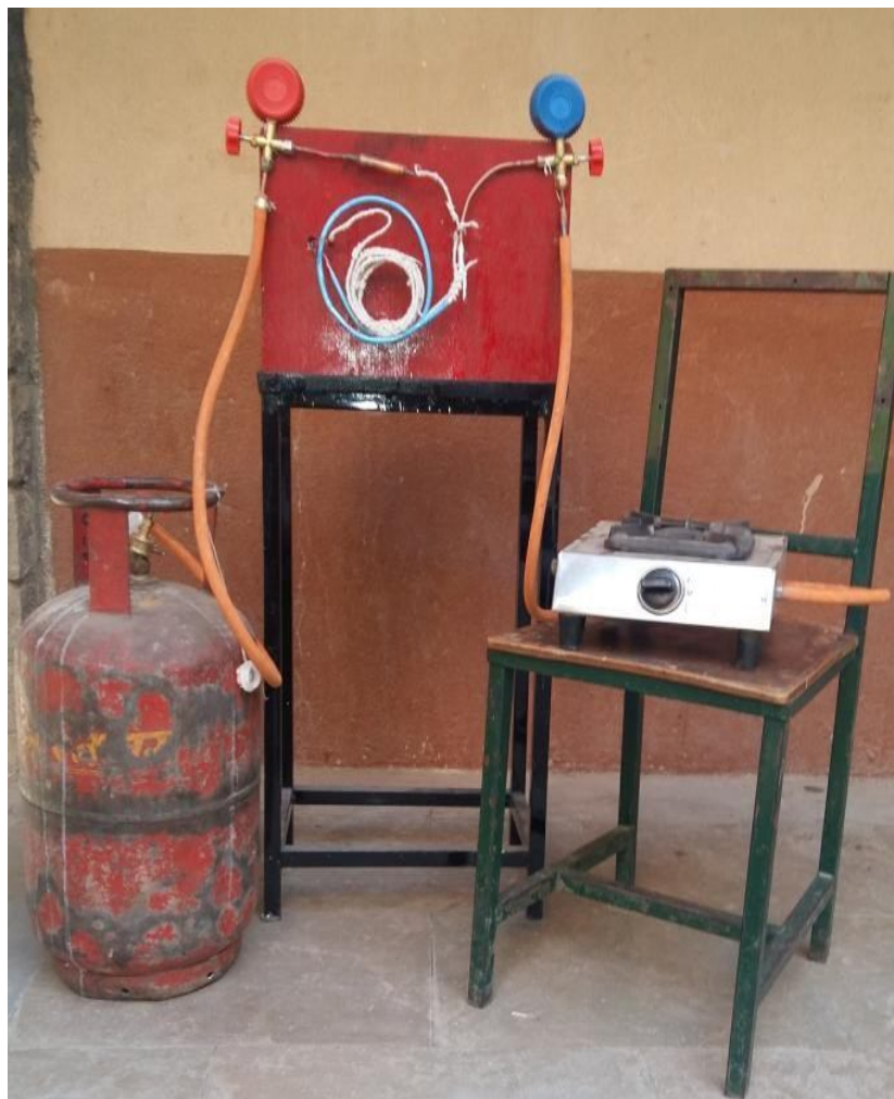
Fig.-3: Actual Setup of LPG Refrigerator
