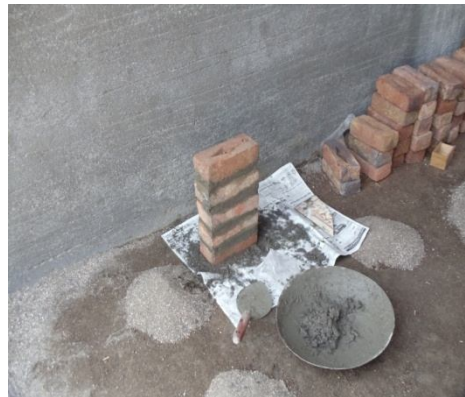
Figure-2: Brick Prism Specimen [Rath, Deo and Ramtekkar (2016)]
