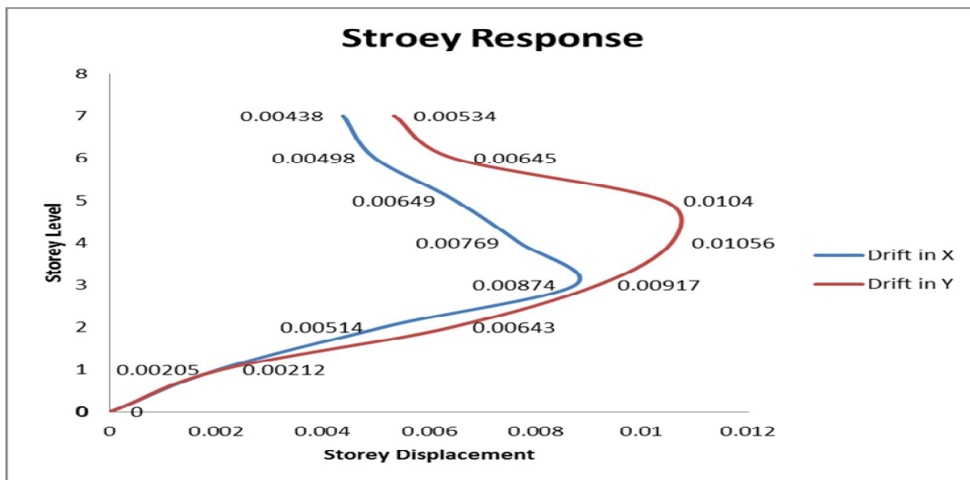
Figure 10. Storey Drift for L.S as performance level low, mid and high rise model
