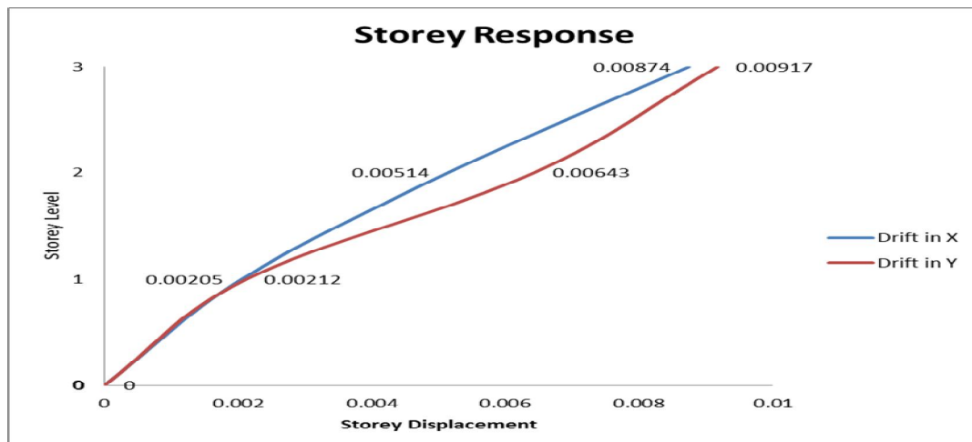
Figure 9. Storey Drift for I.O as performance level low, mid and high rise model
