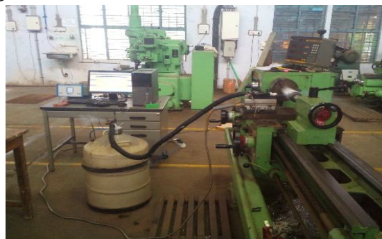
Figure 1: NAGMATI-175 lathe machine with cryocan setup
