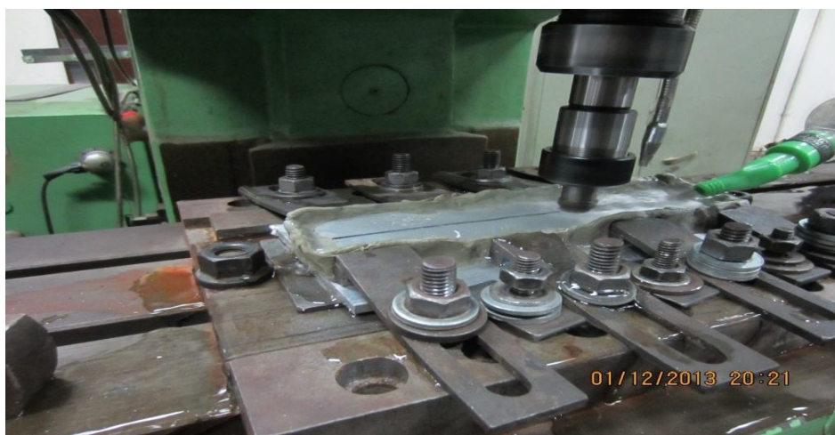
Figure 2 Setup for underwater friction stir welding
