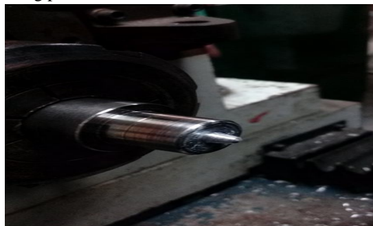
Fig. 4: Tool piece fixed to the rotor
