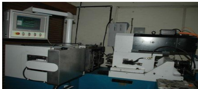
Fig. 2: Friction Stir Welding Machine at IISc
