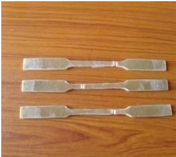
Fig.4 Specimens after Tensile Tests, (a) E- Glass fiber, (b) Carbon fiber
