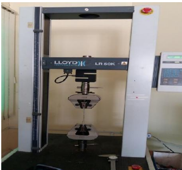
Fig.3 Tensile Experimental Setup, (a) Tensile Test, (b) Compressive Test
