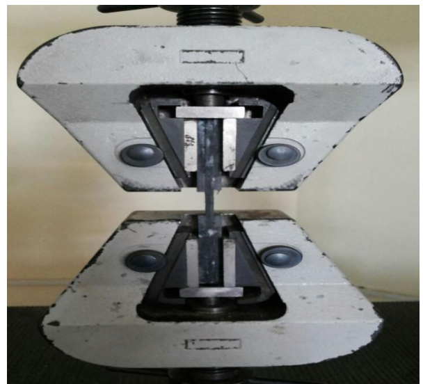
Fig.3 Tensile Experimental Setup, (a) Tensile Test, (b) Compressive Test
