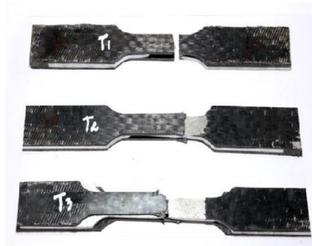
Fig.4 Specimens after Tensile Tests, (a) E- Glass fiber, (b) Carbon fiber
