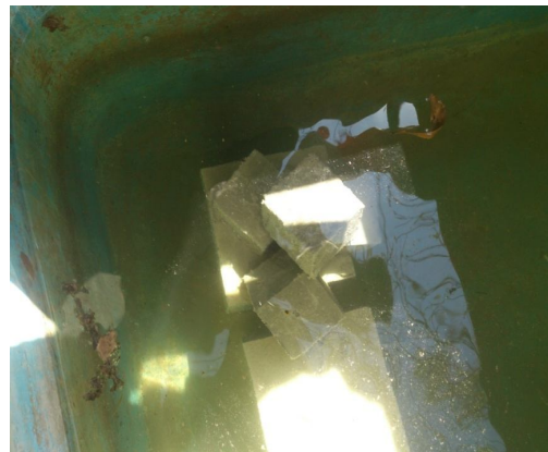
Figure 4(b). Curing of Specimens
