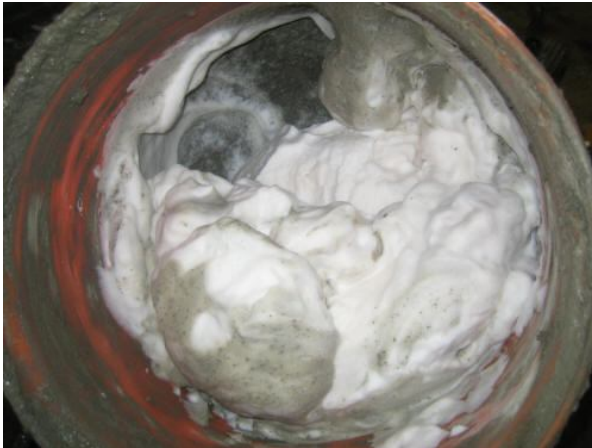
Figure 3(a). Production of Foam Concrete
