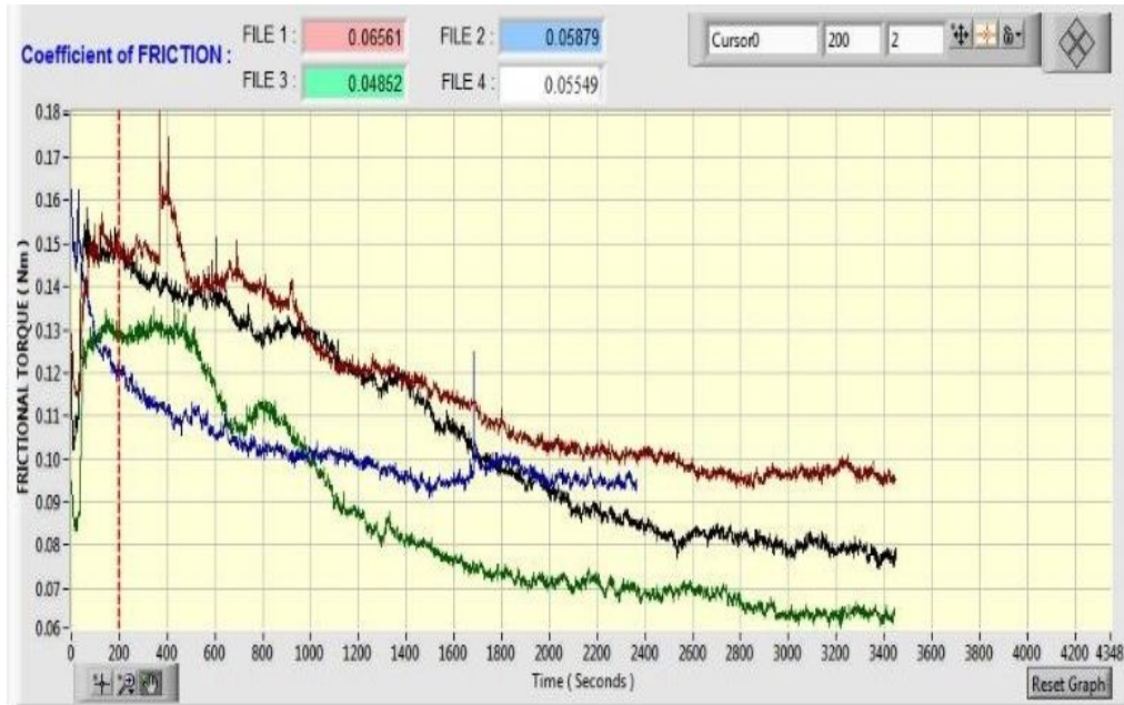
Fig. No. 5 Comparison graph of 0.5%,1% & 2% h-BN nano particles of 0.8 \mu with mahua with Pure Castor oil 65% & Mahua Oil 35%
