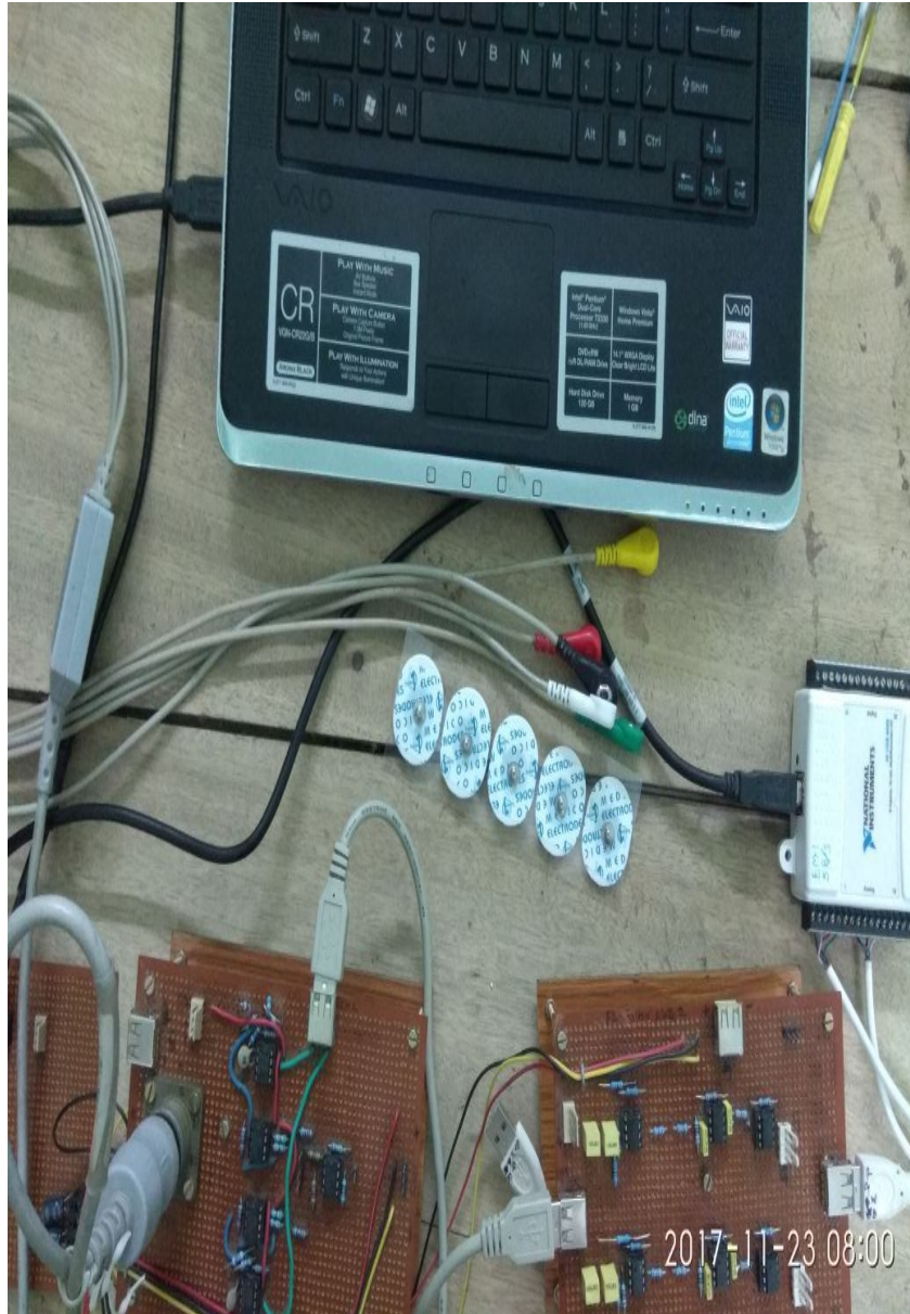
Fig. 6: Setup for Acquiring Speech Related EMG Signals
