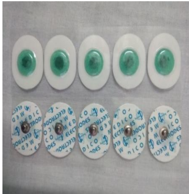
Fig. 3: Typical Surface EMG Electrodes
