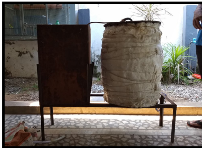
Fig.7 Waste plastic oil extraction set up
