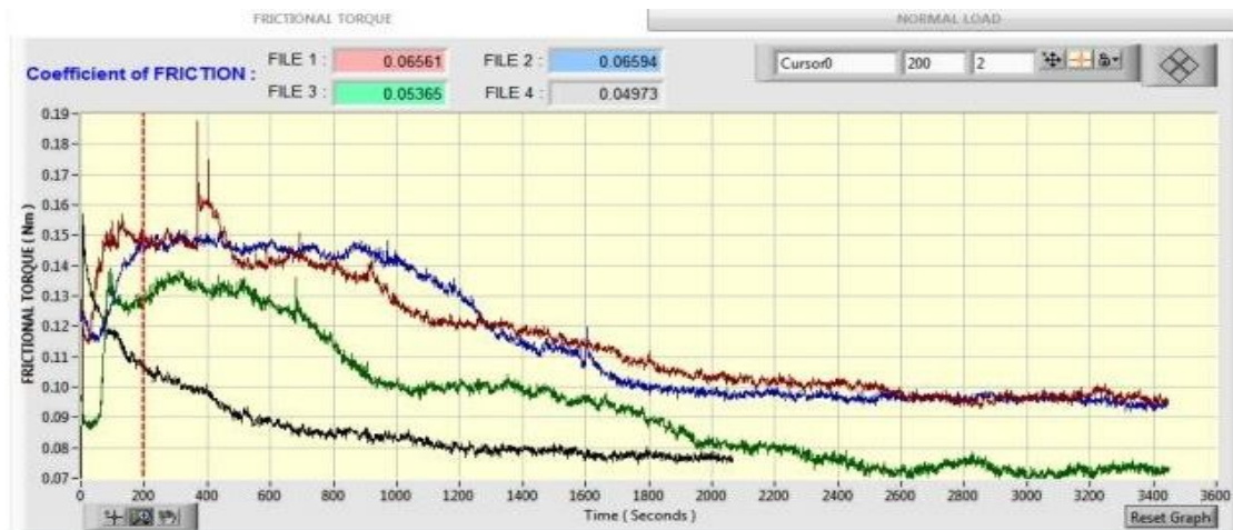
Fig. No. 1 Comparison graph of Frictional torque vs Time for 0.5%, 1% & 2% h-BN Nano particles of 1.5 \mu with Mahua oil 35% + castor oil 65%
