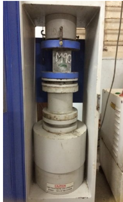
Fig. 3 Concrete cubes M 90 grade specimens in CTM
