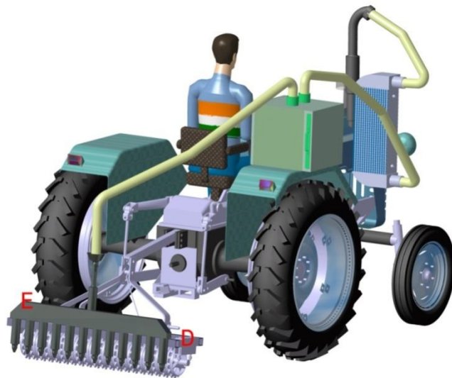
Figure-4 (D- Farming attachment for Tractor, E- Exhaust Injector/ Seeder )
