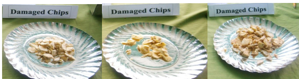
Fig 9. Damaged chips of unripe and ripe bananas and sweet potato. No damaged chips for potato
