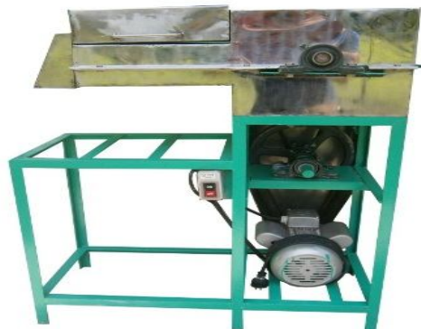
Figure 4. The actual fabricated Power Driven Piston Type Multi - Crop Chipper
