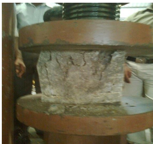
Figure: 4.1 Compressive Strength Test of Concrete
