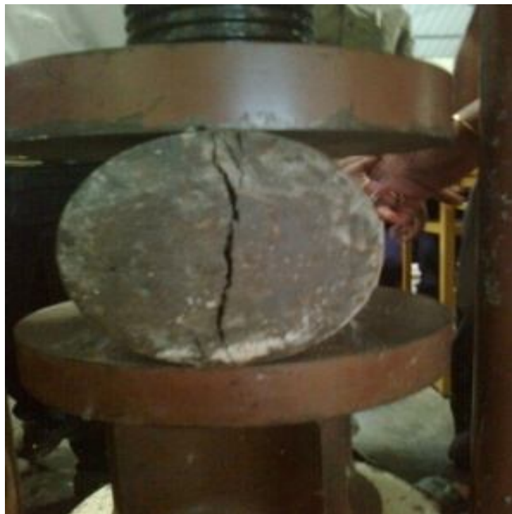
Figure: 4.3 Split Tensile Strength Test of Concrete
