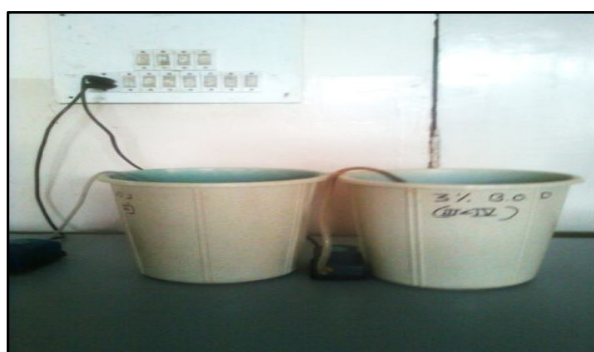
Fig-3: Experimental Set up of SBR
