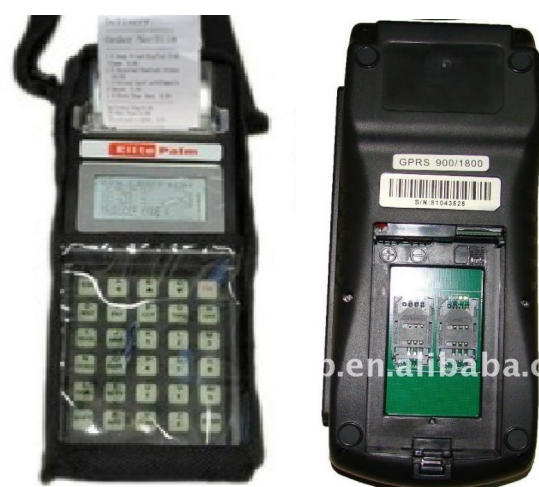
Figure 4. Ticket printer with SIM card slot.
