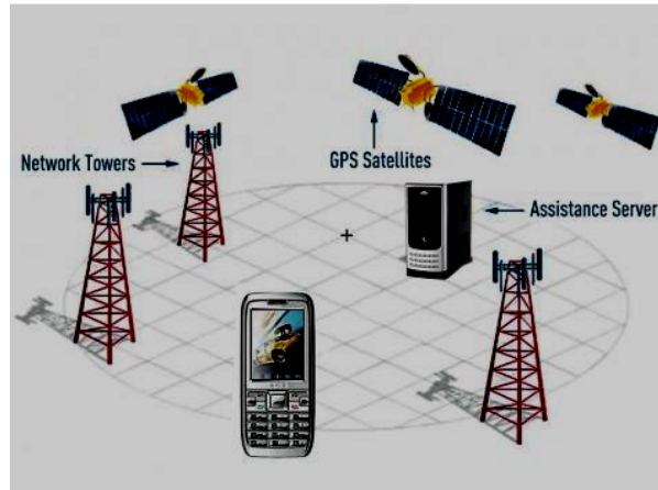
Figure.2.2: Architecture of A-GPS System
