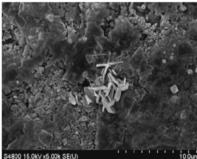
Figure 4: Scanning Electron Microscopy after molding of material with carbon fly ash
