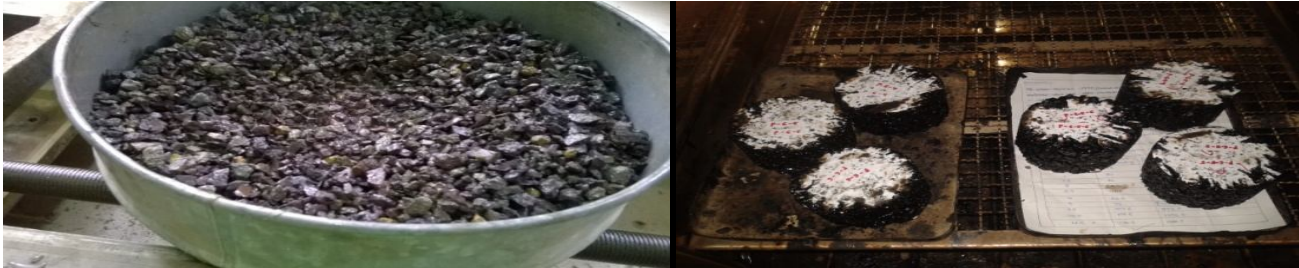
Fig. 1 Steel Slag Aggregate and Samples prepared for Marshall Test
