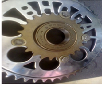
Fig.9. 48no.Tooth sprocket mounted on wheel.
