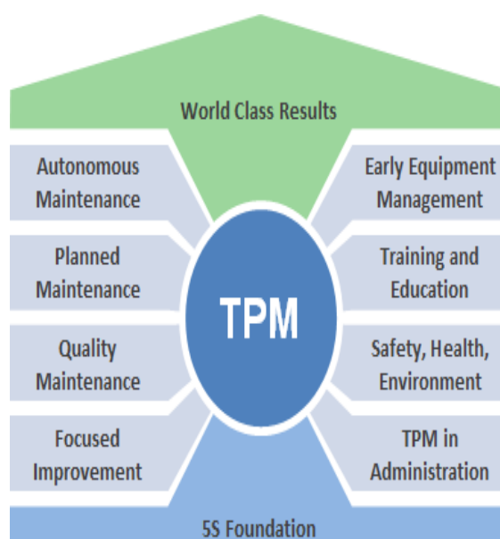
Fig.2 The traditional TPM model consists of a 5S foundation (Sort, Set in Order, Shine, Standardize, and Sustain) and eight supporting activities
