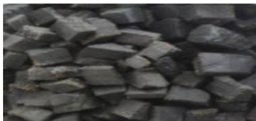
Figure 1: Discarded Rubber tyre pieces of size 1cm x 2 cm used as aggregate in concrete specimens.
