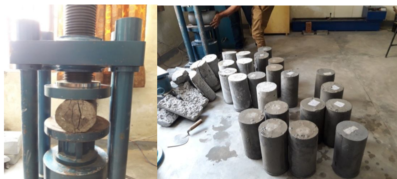
Figure 3: Split tensile strength test of cylindrical specimen with different composition.
