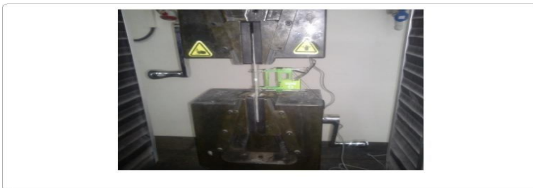
Figure 2:Tensile test set-up.
