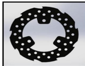
Figure 28: CAD of 240mm Dia. Rotor
