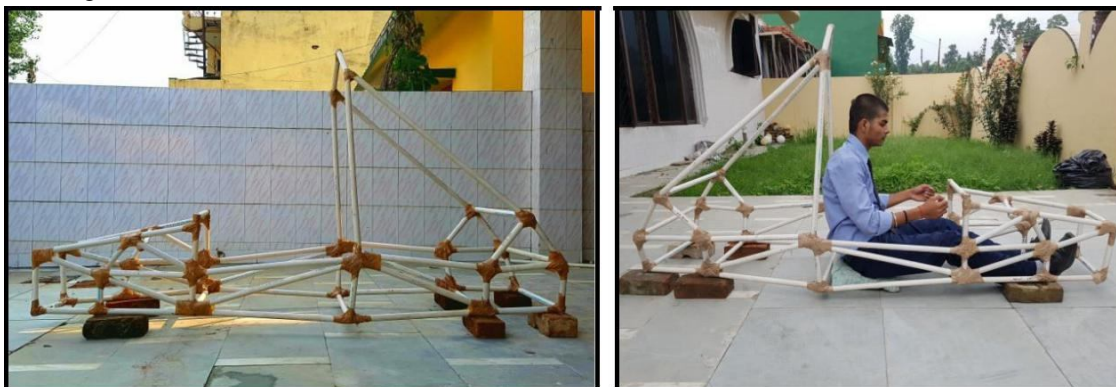
(a) PVC tube model (b) Re-dimensioned PVC tube model Figure 3: PVC tube models of the frame design
