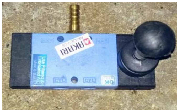
Fig 2: Direction Control Valve
