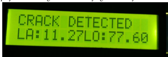
Fig 8: LCD Display When Crack is Detected
