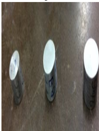
Figure 10 compacted sample of Al-6063
