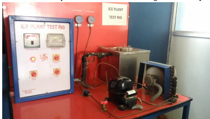
Figure 1. Test rig of vapour compression refrigeration system
