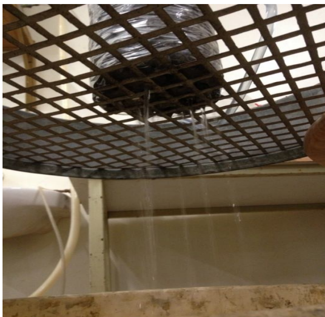
Fig.1 Water passing through the pervious concrete specimen during permeability test
