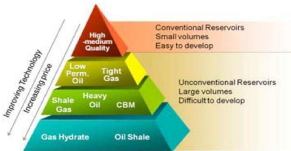
Fig. 3 - Resource triangle shows majority of available resources will require improved technology to recover (Dong et al. 2011).
