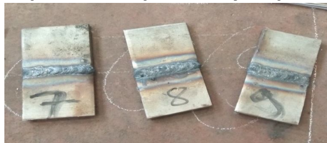
A.80Amp(50° angle) B.90A(60° angle) C.100A(70° angle)
