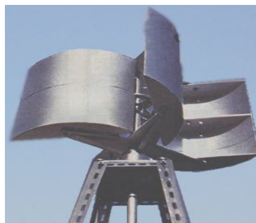
Fig 3b Savonius model
