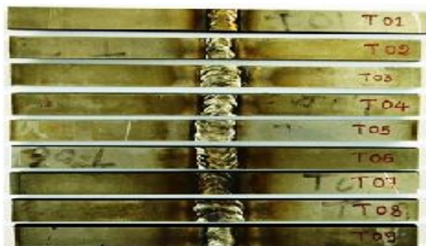
Fig. 7 Impact test specimen
