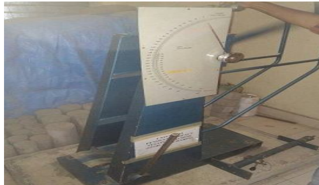
Fig. 6 Impact testing machine
