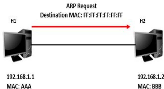
Fig 2. ARP Request (Broadcast Request)
