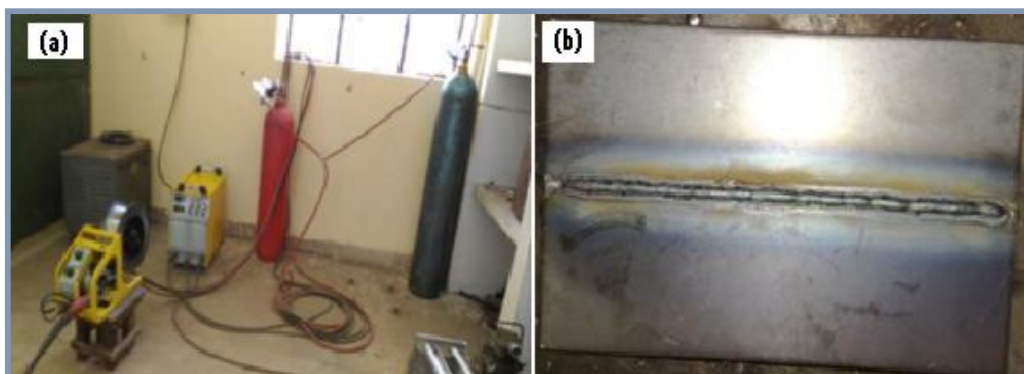
Fig. 1. (a). MIG welding setup, (b). Welded component.
