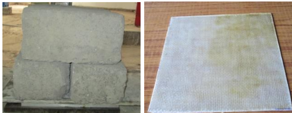
Fig 2: Weight on the mould cavity, E-Glass laminate
