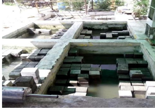
Figure 2- Casting of cubes and curing tank
