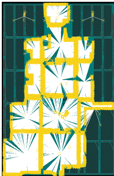
Fig 4 Clock Gate Cloning done using K means clustering
