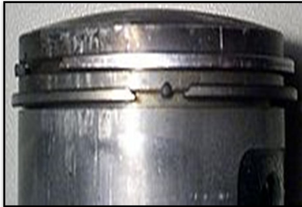
Figure 1. A pair of piston rings mounted on a two-stroke cycle scooter piston
