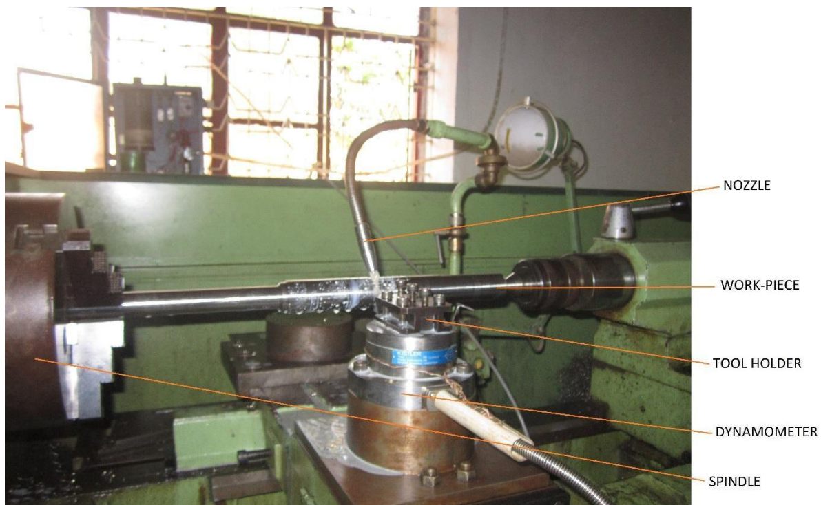
Figure 2.2: Experimental setup for MQL lubrication system
