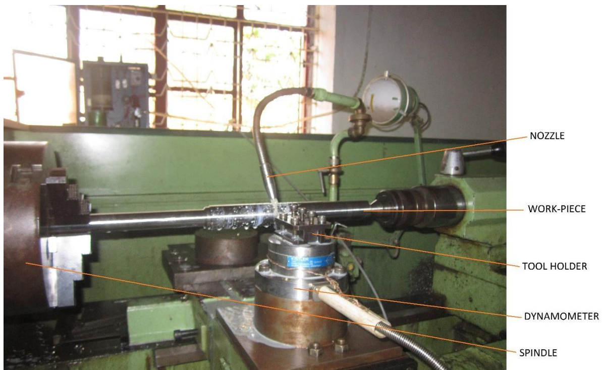
Figure 2.2: Experimental setup for MQL lubrication system
