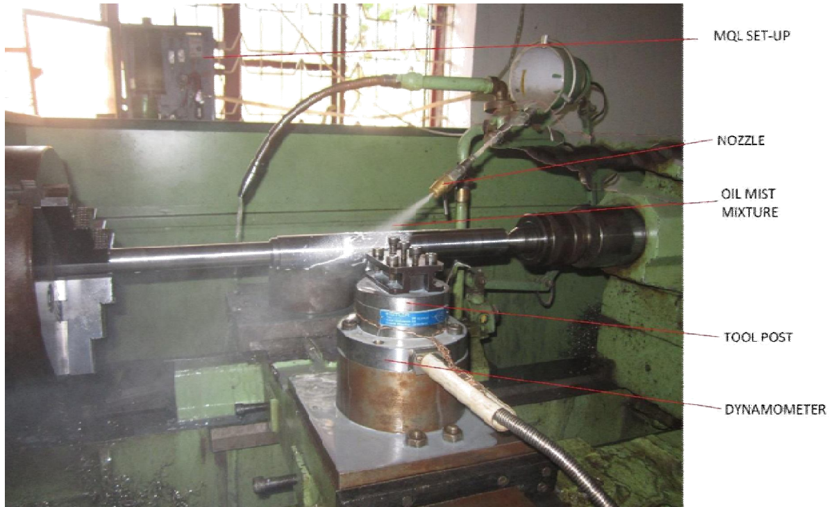
Figure 2.1: Experimental set-up for conventional cooling
